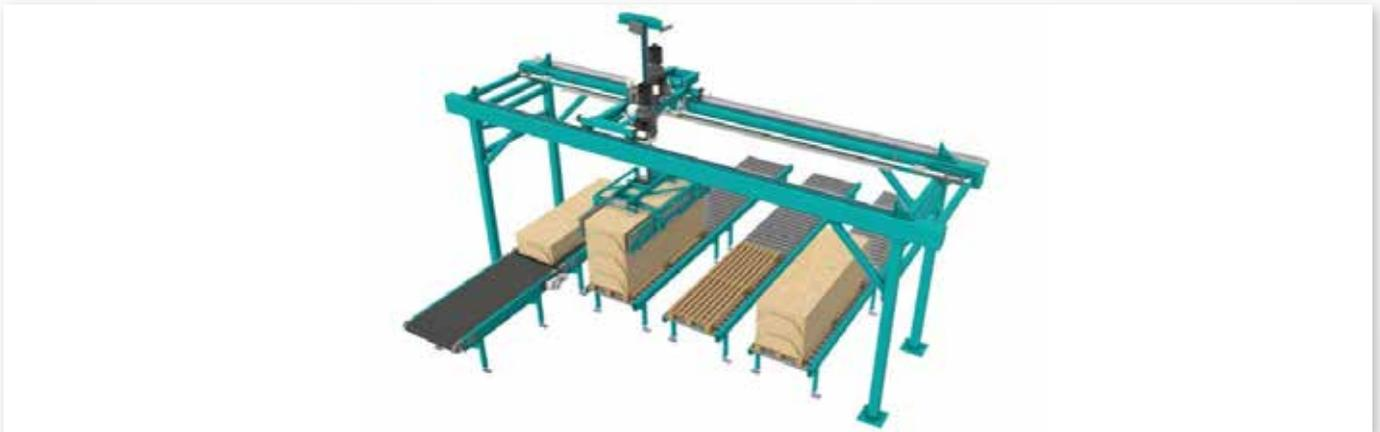
The product dimensions, shapes and weights are the basis for the selection of the conveyor type, together with capacity required, and if change of conveyor direction is required.
